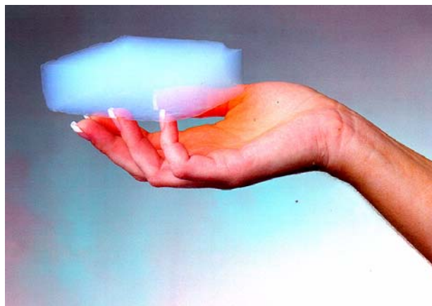
Figure 4: A silica aerogel is virtually made of air (up to 99,5 %), Source NASA.
