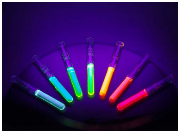
Figure 10: Nanoparticles (CdSe particles, diameter 3-6 nm) with different diameters fluorescing under UV light. Flad & Flad Communications
