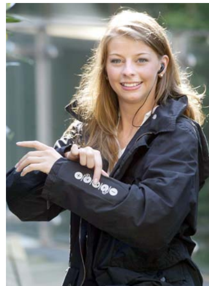
Figure 12: A jacket with „wearable electronics“. A MP3 player and keyboard on the sleeve has been embedded. Rosner GmbH + Co.
